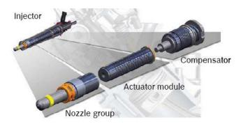
Fig. 6. Main modules of the GDI piezo injector
