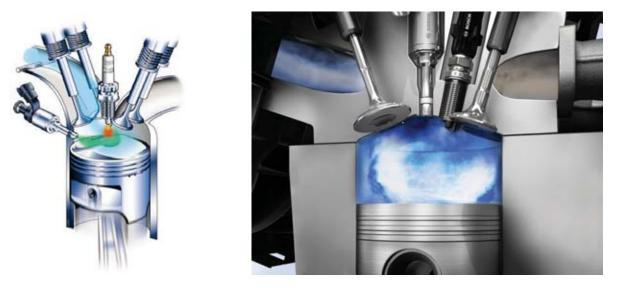
Fig. 1. Wall-directed combustion system
