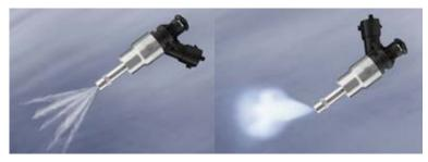
Fig. 5. The spray shapes of the GDI solenoid injectors
