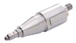
Fig. 19. HyICE High pressure (late injection) DI: solenoid actuated needle injector; injector characteristics; flow area: 1 mm2, pcyl.max: 180 bar, pH2max: 250 bar
